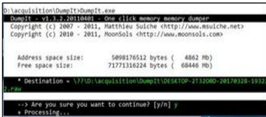
Figure 4. Acquisition Process Using DumpIt
